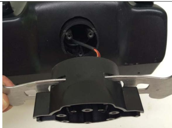
10. Install the adapter base puck by aligning the notches on the puck with the tabs on the base shaft. Then press the puck on to the base shaft.
