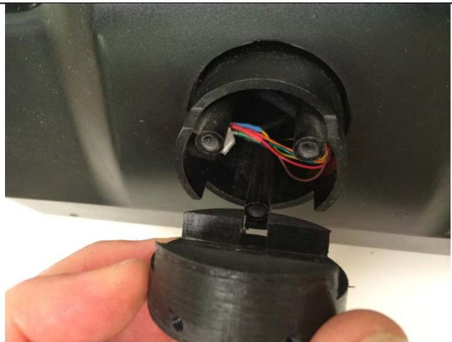
11. Install the three #10 x 1 ½" (38mm) self-taping screws ensuring the base puck tightens down flat onto the base shaft.
